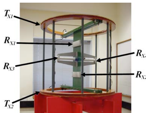
Figure 3. The transmitter-receiver section of the EM ELF gradiometer. Tx1, Tx2 – transmitter loops wound on circular wooden frames with 1.4 metres in diameter, 100 turns each. The typical operation current is 10 A peak. Rx1, Rx2, Rx3, Rx4 – receiver coils.
