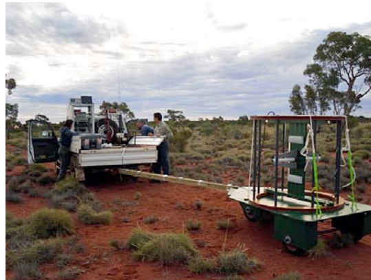
Figure 4. The EM ELF gradiometer field trial with Regis Resources Pty Ltd commenced in July 2009
